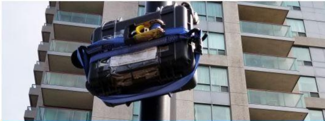
Noise logger capturing ambient noise
