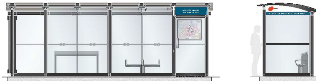
12m by 2m Enhanced Shelter
