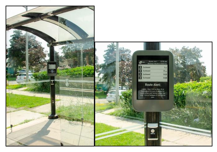
The 10-inch reflective, solar-powered, LCD model, displays information in colour. When you push a button below the screen the display changes to a high-contrast version with larger text. The screen is installed at bus stop #0661 located at Central Parkway West at Semenyk Court, which serves Routes 6 Credit Woodlands and 38 Creditview.
