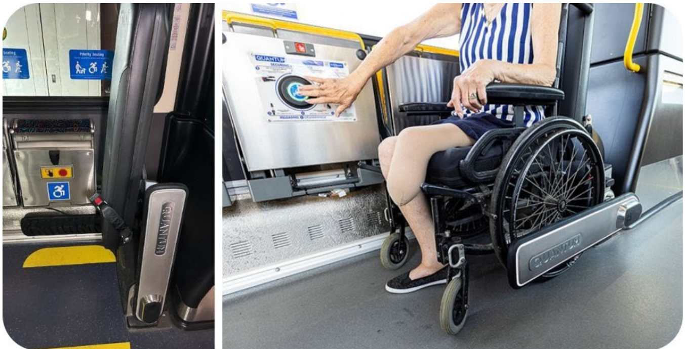
Figure 13: Example of Q-Straint system installed on a bus and being used by a customer in a wheelchair.
